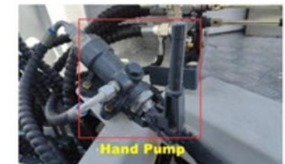
6. Hand Pump: when there is something wrong with truck chassis, or the electric system not working, use this Hand Pump to release the pressure, then can reposition the aerial platform truck
